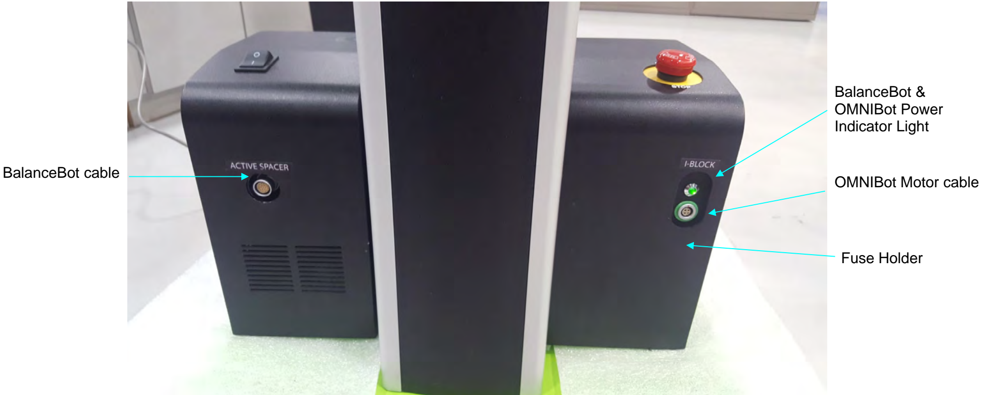
Enclosure Box connections – Front View
